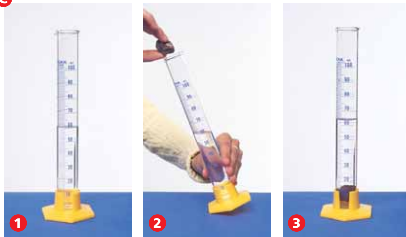
Measuring the volume of an irregularly shaped solid
