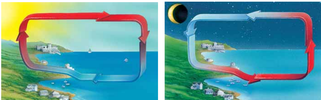
Figure 10.30 Sea breezes can be felt as far as 70 km from the coast (A). At night, convection currents reverse and an offshore breeze blows out to sea (B).
