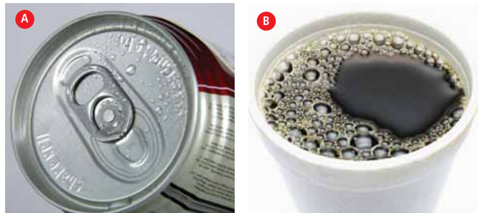
Figure 10.7 Aluminum is a good thermal conductor (A). Styrofoam® is a good thermal insulator (B).
