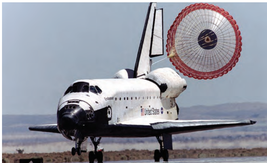
Figure 9.8 A parachute reduces the landing run of a space shuttle, reducing wear on the brakes and providing increased directional stability.
