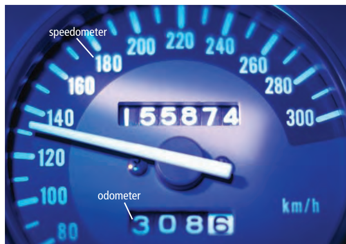
Figure 8.4 The odometer displays the distance the car has travelled. A speedometer indicates the car’s speed.
