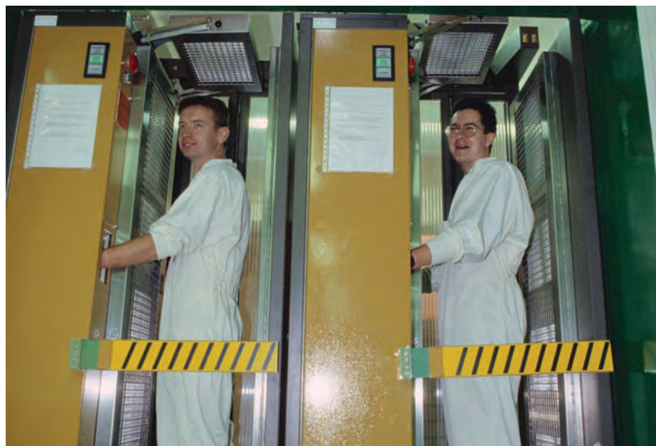
Figure 7.18 If you visit a nuclear energy facility, you might find yourself standing in one of the devices shown above. This full-body scan detects whether the radiation levels of the workers exceed safety standards.
