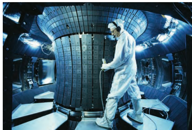
A technician performs maintenance on the doughnut-shaped device that confines hot plasma.
