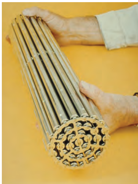
Figure 7.25 Each CANDU fuel bundle is about 50 cm in length and 10 cm in diameter and generates about 1 million kWh of electricity during its time in the reactor.
