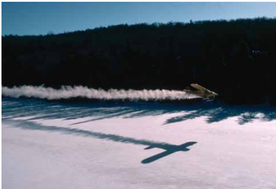
Figure 5.17 Adding lime to a lake
